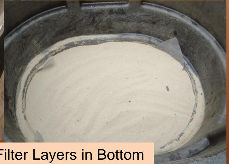
Gravel Drainage and Sand Filter Layers in Bottom
