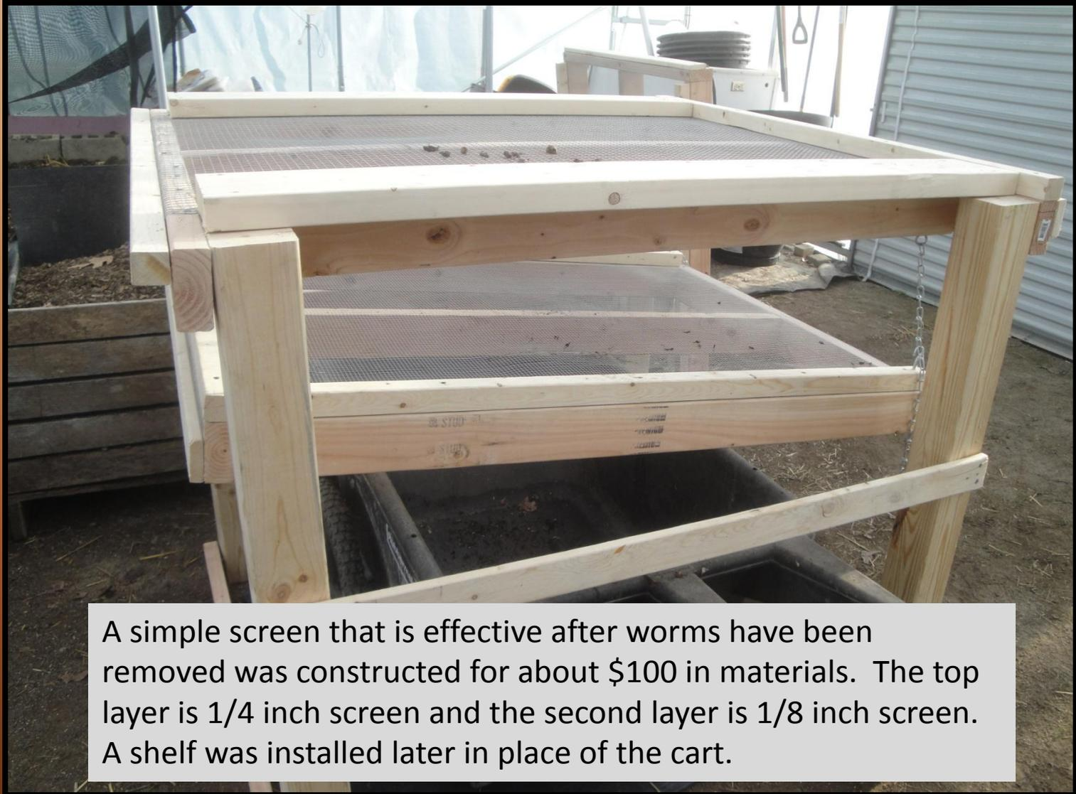
A simple screen that is effective after worms have been removed was constructed for about \$100 in materials. The top layer is 1/4 inch screen and the second layer is 1/8 inch screen. A shelf was installed later in place of the cart.
