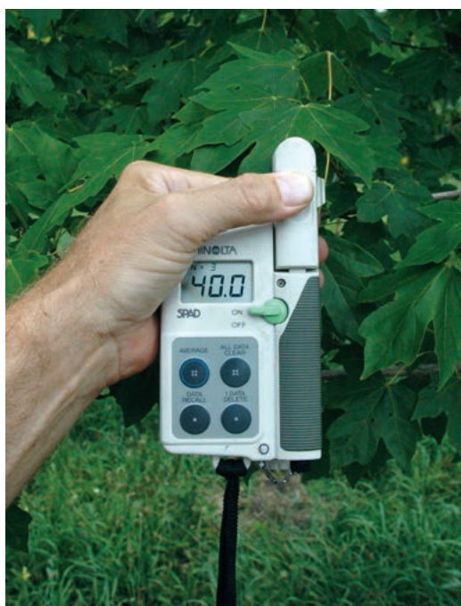
Photos 2 & 3. SPAD index can provide a rapid means to assess trees with high (Photo 2) and low (Photo 3) nutrient status.
