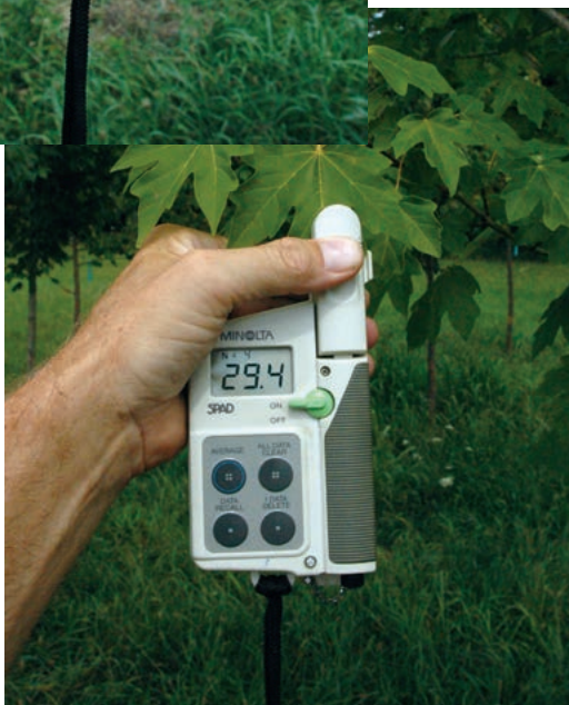
Photos 2 & 3. SPAD index can provide a rapid means to assess trees with high (Photo 2) and low (Photo 3) nutrient status.
