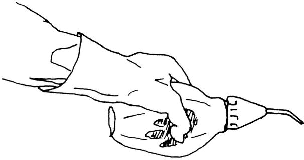
**Plunger dusters** hold more dust than the first two hand-held dusters discussed. Plunger-type dusters have been used for garden dusting for a century, but the plunger duster used in structural pest management is smaller, made of high-impact plastic, and has several styles of nozzles.
