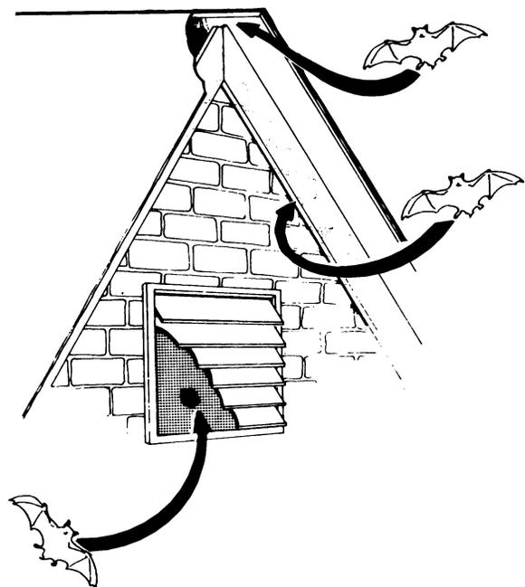
**Figure 19.3.** Common entry points for bats in a building.
