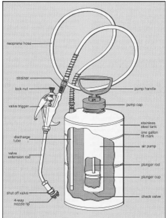
Figure 2-2. The major parts of a compressed-air sprayer (Provonsha).
