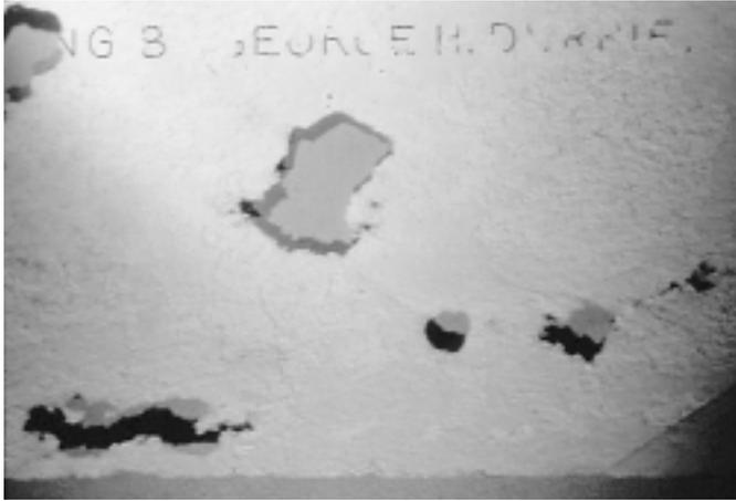
Figure 9.2. Silverfish damage.
