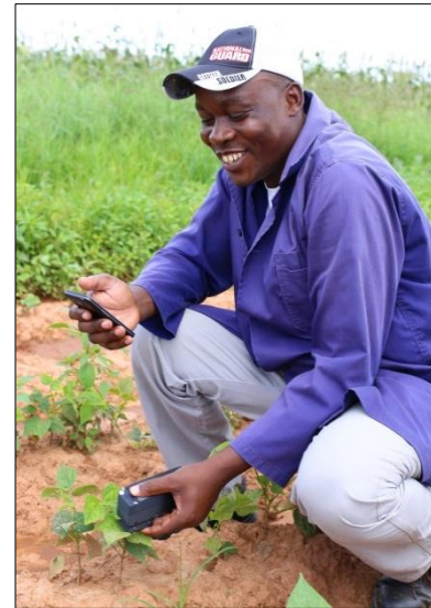
A member of Dr. Kamfwa's team takes photosynthesis readings of a bean plant using the MultispeQ.
