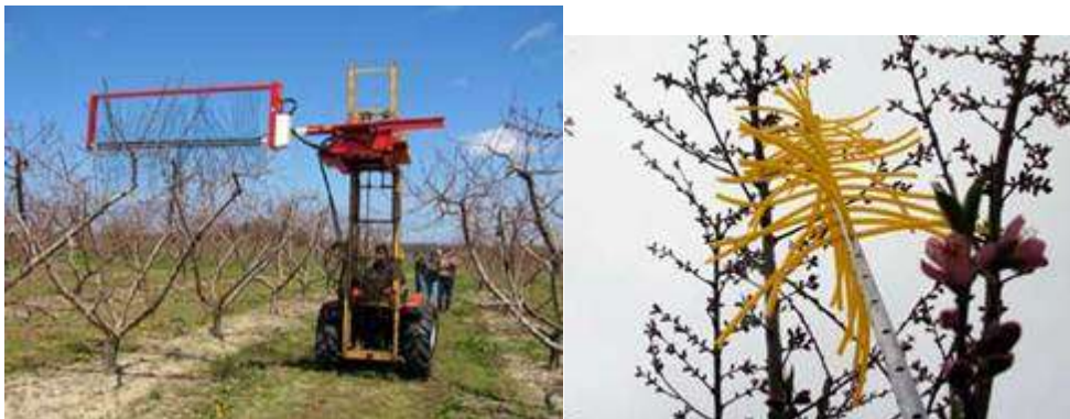
Left - The Darwin PT250 blossom thinner on a lift tractor can reach sides and tops of peach trees.
