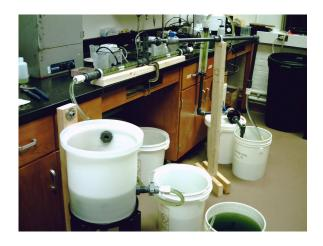
The flocculated algae are then allowed to concentrate via settling, and then dewatered via filtration.
