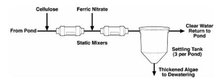
The flocculation process agglomerates individual micro-algae cells into macroscopic entities which are easily dewatered through settling, filtration, and pressing. Our two stage flocculation process starts with addition of ferric nitrate, followed by addition of cellulose fiber, and produces a fibrous floc which withstands the shear forces of dewatering.
