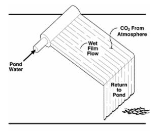
Another contacting option would be to provide a ramp above the pond, at the top of which a portion of the pond water would be pumped so as to provide a thin film of water flowing down the surface of the ramp, where the water would absorb atmospheric carbon dioxide at a higher rate than in the pond itself. We budgeted 1 kW of pumping power for this analysis.
