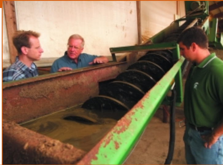
Wallace, Bickert and Kirk watch the sand-manure separator as it works to separate liquid manure and sand. Once heavy sand is removed, the manure can be stored and used as a nutrient source.
