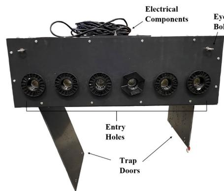
Figure 5: Final trap design (side view)
