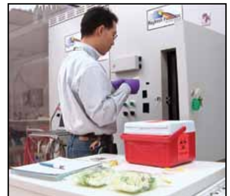
Sanghyup Jeong, a visiting assistant professor in biosystems engineering, loads samples of lettuce into a prototype x-ray device to kill bacterial pathogens. (Photos by G.L. Kohuth)
