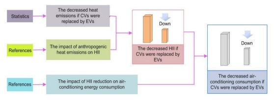
Figure 3 | Diagram of the methods. The data source and procedure of reasoning and estimating are presented. CVs, conventional vehicles; EVs, electric vehicles; HII, heat island intensity.
