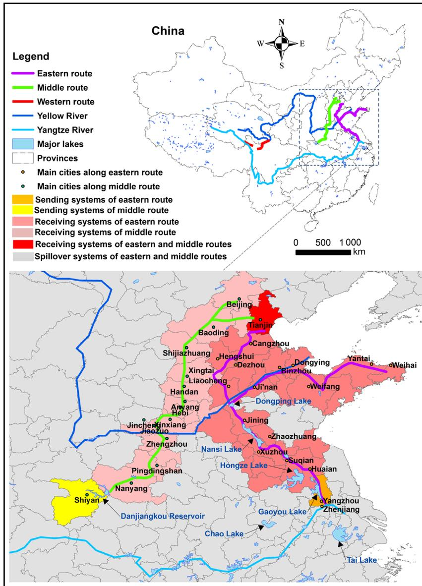
**Figure 2.** A schematic diagram of the South–North Water Transfer Project (SNWTP). The lower part of the figure (inset map) highlights the sending, receiving, and spillover systems, as well as the main cities located along the Eastern and Middle routes. Many spillover systems such as those outside of China are not shown.
