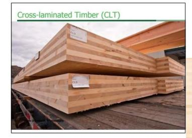
A structural panel consisting of three, five, or seven layers of dimensional lumber that are able to bear loads in and out of plane, which can be used as floor or wall system.
