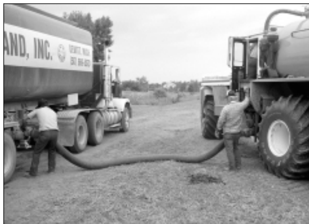
Liquid biosolids are transported to agricultural fields by large tankers and then transferred to applicators for injection into the soil (Benton Harbor–St. Joseph land application program).
