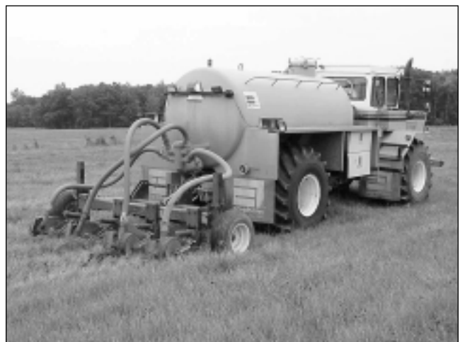
Liquid biosolids can be applied to grass or forage crops with minimal soil disturbance using special sod injectors, such as this injection unit in use at Port Huron, Mich.
