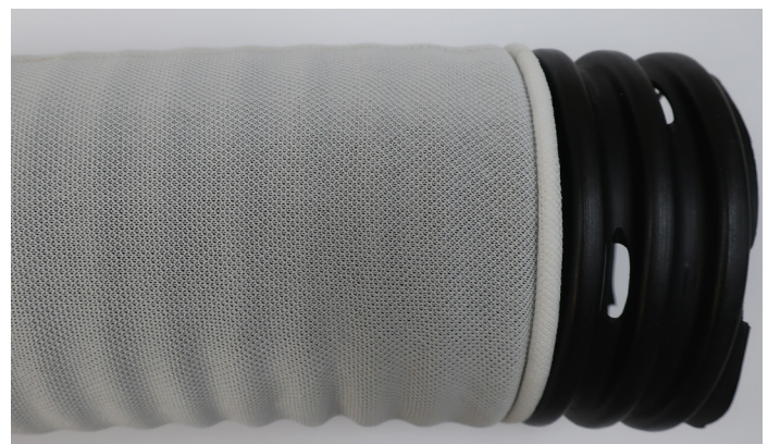
Figure 5- A muck pipe wrapped with a knitted sock envelope. The muck pipe has large oval perforations that reduce the chance of iron ochre clogging compared to narrow slotted pipes.
