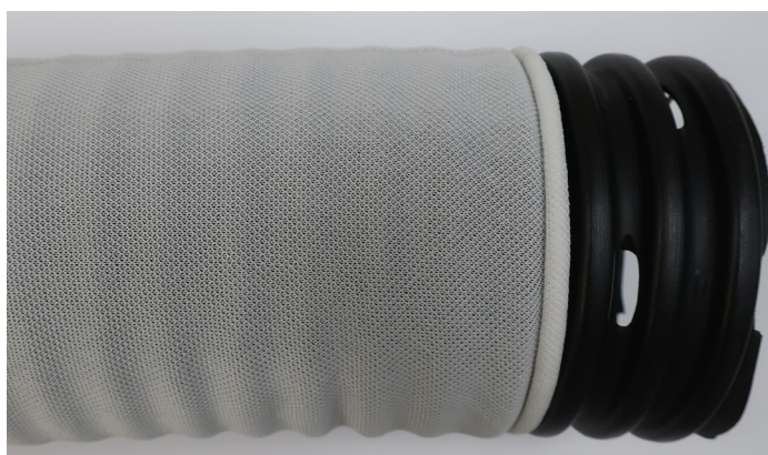
Figure 5- A muck pipe wrapped with a knitted sock envelope. The muck pipe has large oval perforations that reduce the chance of iron ochre clogging compared to narrow slotted pipes.
