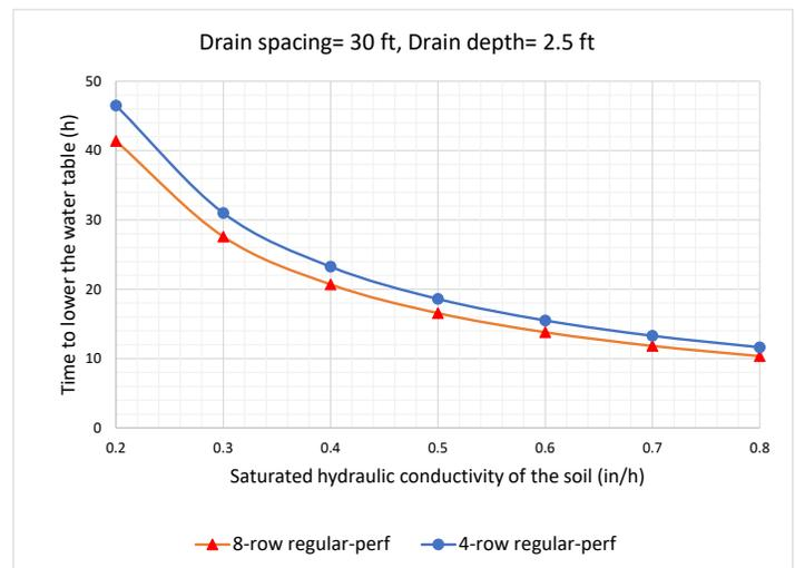
Figure 3- An 8-row regular-perforated pipe lowers the water table from the soil surface to 1-ft depth, 11% more quickly than a 4-row pipe, when installed at 30-ft spacing and 2.5-ft depth. Drainable porosity is 0.04 and depth to restrictive layer is 6.5 ft.
