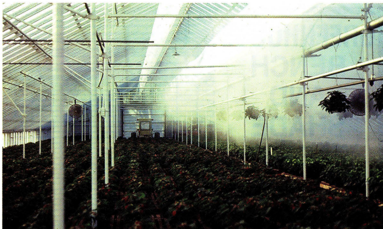
Airflow pattern can be checked with fog or a smoke bomb. The air should flow continuously down one side of the greenhouse and back up the other at a rate of 50-100 feet per minute without short-circuiting.
