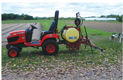
Versatile equipment is an economical means to get the job done with less labor. A sprayer for vegetable production allows liquid nutrient solutions such as fish emulsion or compost tea to be evenly applied to a field. Sprayers are also useful to apply OMRI approved pesticides. Note the versatility of this sprayer with a hand boom, which can be used to spray fruit trees or brambles.
