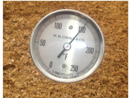
**Figure 2. Long-stem thermometer used to monitor internal temperature. (credit: T. Guthrie.)**
