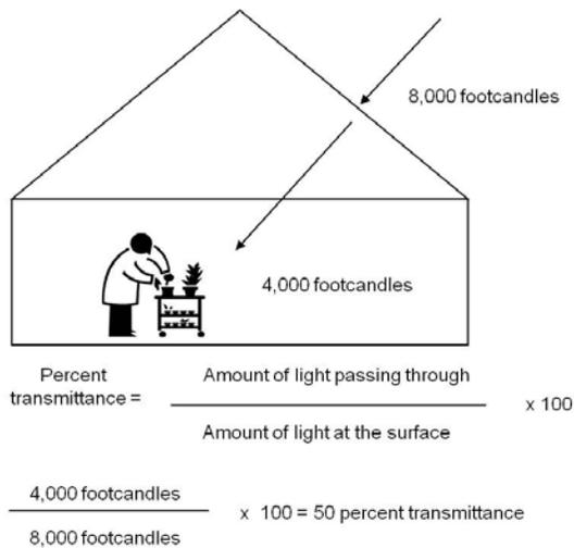
Plastic / polyethylene greenhouse plastic film light transmission will decrease over a period of years. Measuring light transmission is one of the best ways of testing when to replace the film.
