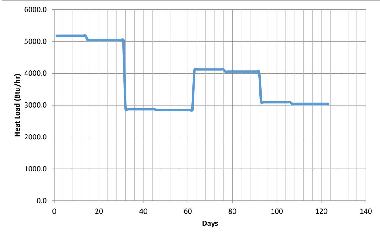
*Figure 2: Heat load from August to November without the field heat*
