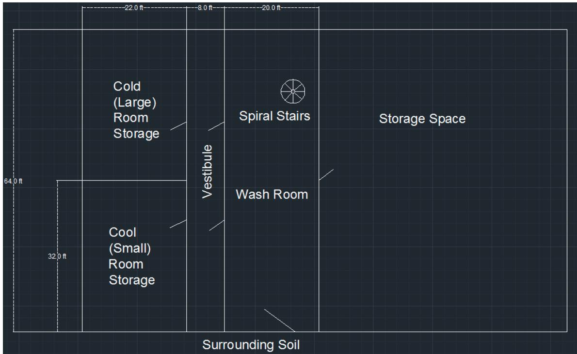
*Figure 7: Plan View Cold Storage Basement*
