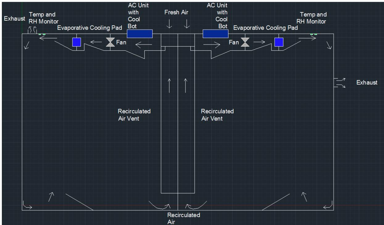
*Figure 9: Plan view of the ventilation system*
