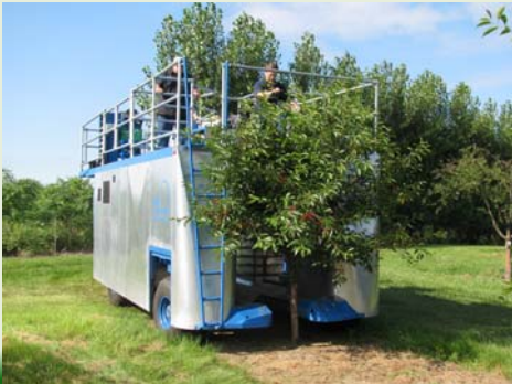
BEI 3000 Tested July 2010 Rotary-Tine Tower harvester tested at Cherry Bay Orchards, Hartford, MI of 4 yr old Monts.
