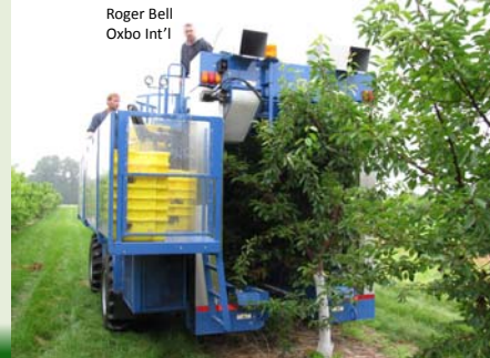
Oxbo 9000 Tested at CRC July 2009 proved effective and efficient in harvesting MSU tart selections, seedlings and Monts in bush form, without damaging trees
