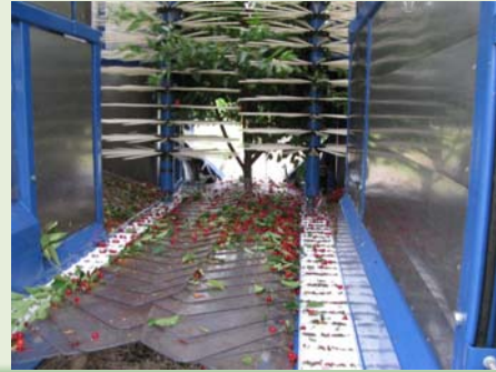
Oxbo 9000 Tested at Wright Orchard, Belding, MI July 2009 Rotary-Tine Tower Mechanism
