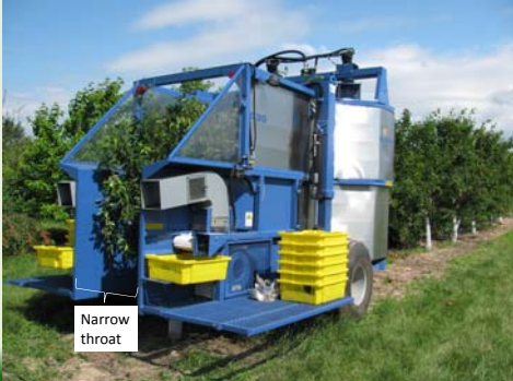
Oxbo 930 Tested at CHES July 2009 proved too narrow thresh hold and aggressive... severe damage to trees
