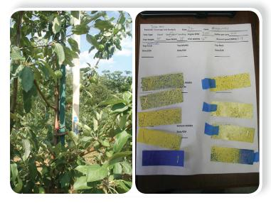
Left: Water and oil-sensitive paper was hung in this highdensity planting by dividing the canopy into nine zones and using furring strips to locate the paper in through the canopy. **Right:** Overspray is observed where watersensitive paper turned completely blue and can result in pesticide sheeting off the leaf surface. Peter Werts/IPM Institute of North America, Inc.
