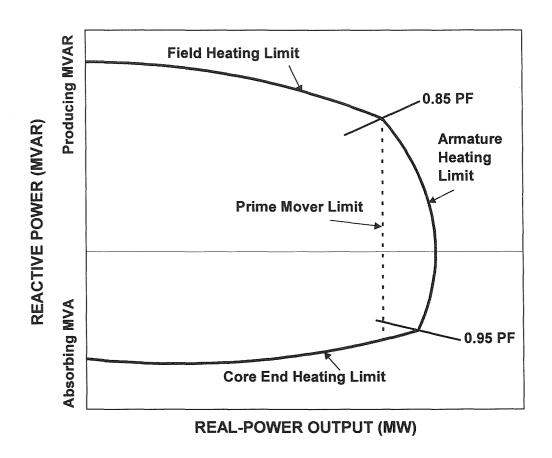
Figure 7-3. Reactive-power capability depends on real-power production for a synchronous generator.
