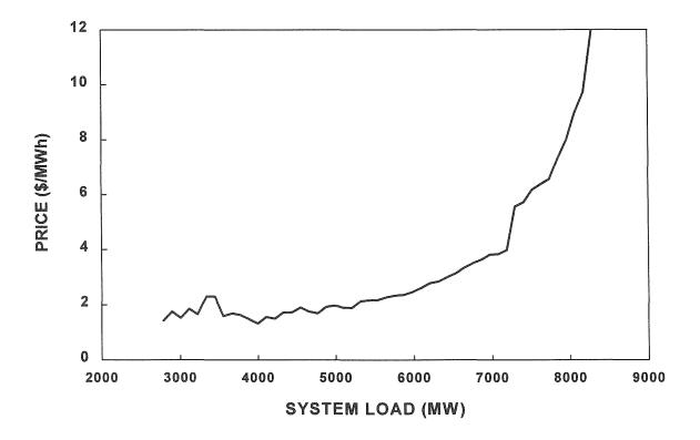
Figure S-1. The cost to consumers for eight generation-provided ancillary services as a function of system load for a hypothetical utility system.
