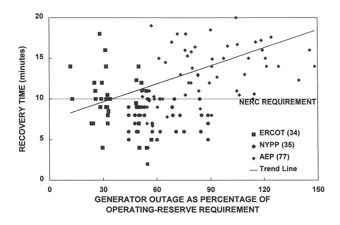
Figure 5-3. Time to recover from a generator outage as a function of the outage magnitude relative to the minimum reserve requirement for three systems.
