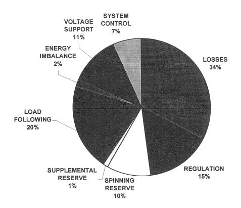
Figure 4-1. The allocation of ancillary-service costs for a hypothetical system. (In total, these services cost the equivalent of \$2.3/MWh during the course of a year.)
