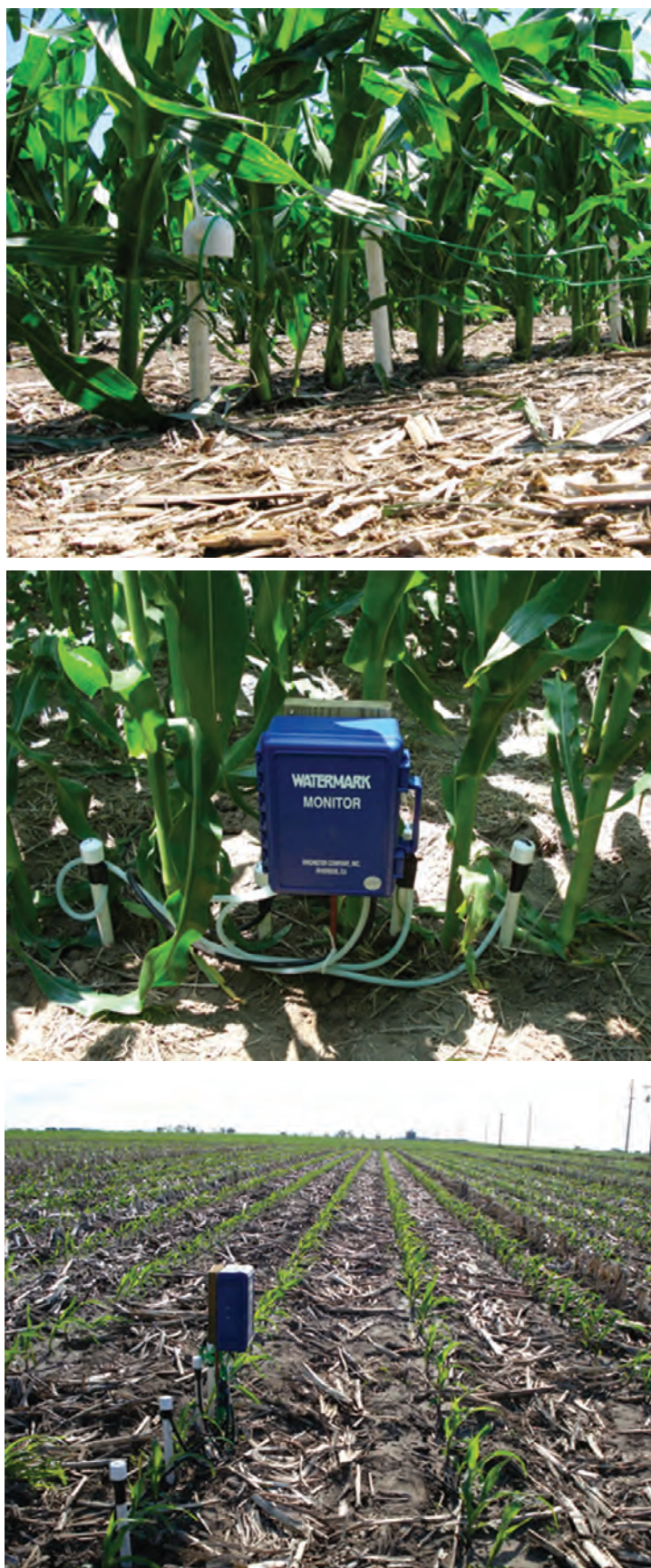
Figure 5. Typical installation of Watermark soil moisture sensors in various corn fields.
