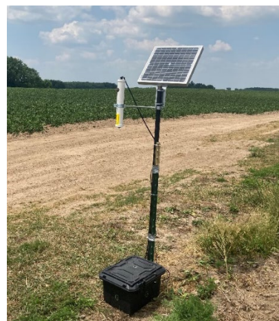
Fig. 1. Rotating arm impactation sampler deployed in a commercial potato field in 2023.
