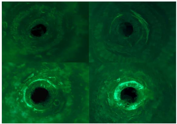
Figure 6.—Example of the subjective OTC mark ranking scale (poor mark—upper left; fair mark—upper right; good mark—lower left; and excellent mark—lower right).
