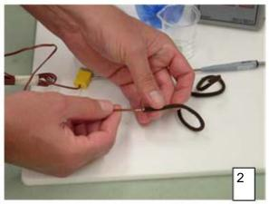
wish to purchase wicks commercially, such as from an online supplier (<u>http://www.wickstore.com/wetbulbwick.html</u>), or a good substitute is a round cotton bootlace (image 2). See page 51 for more information on supplies for a wet bulb thermometer.
