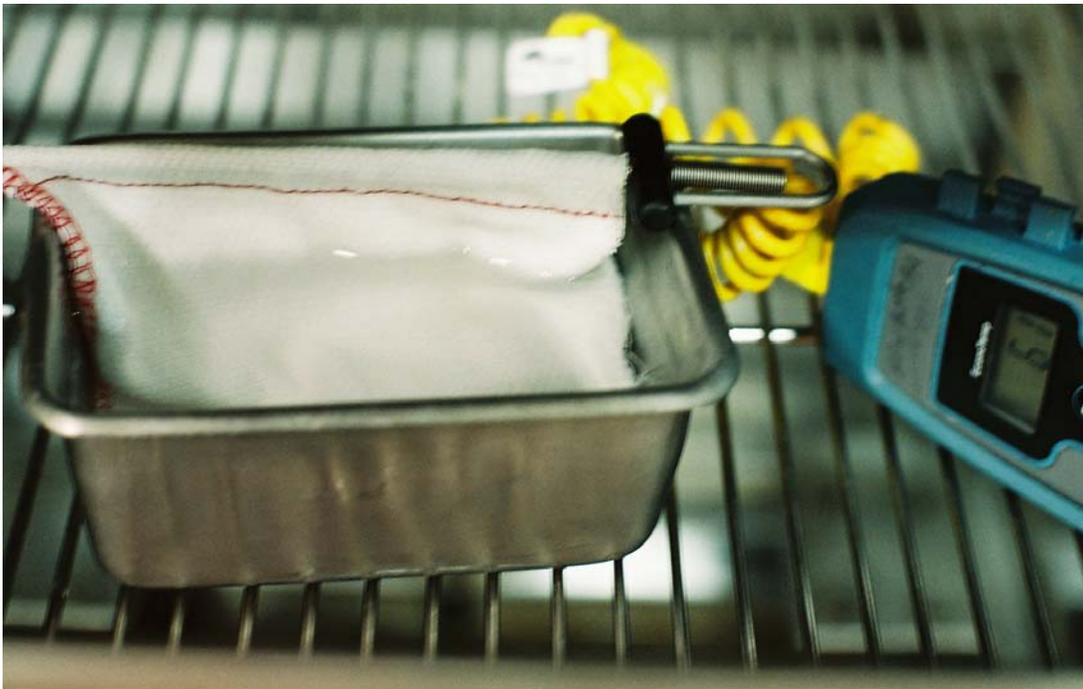
A wet-bulb probe needs to be placed close to the exhaust damper, and so that air can pass over the wet sock as it leaves the oven. Most engineers agree that the air at the exhaust damper is most representative of the condition of the air in the oven.
