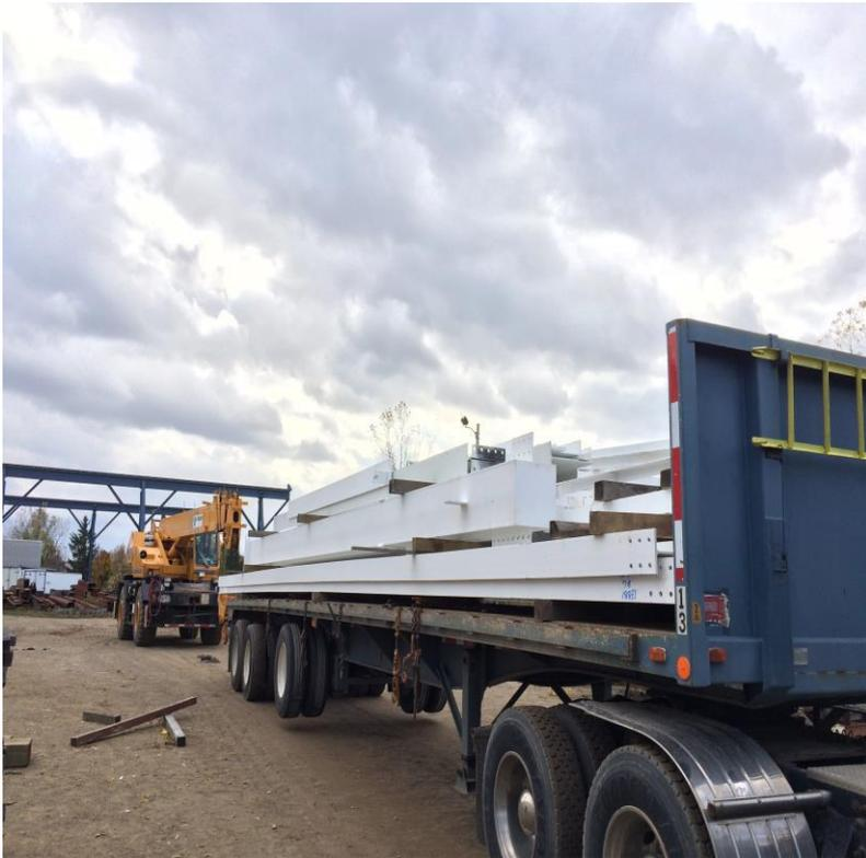
Fabricated shapes loaded and ready for shipping
