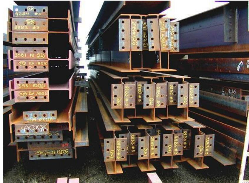
Fabricated beams ready to be shipped
