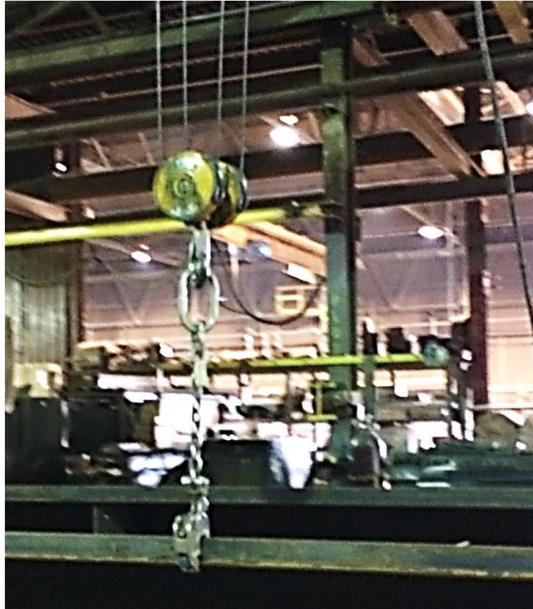
Overhead crane, chain, hook and hardware used to move beams during fabrication
