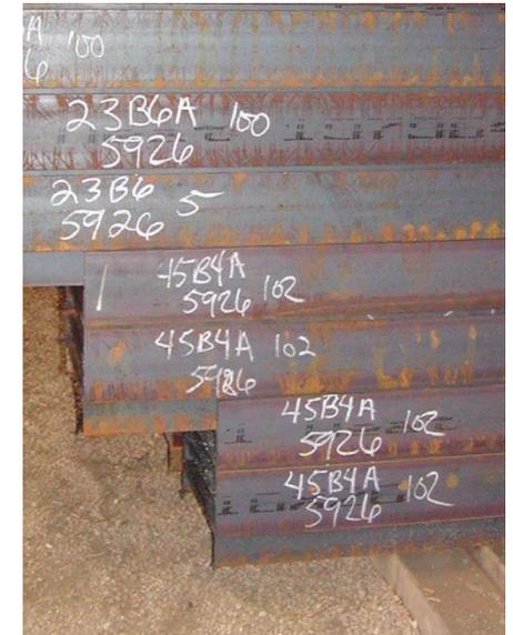
The variety of raw and fabricated steel shapes at the shop require planning and care when stacking
