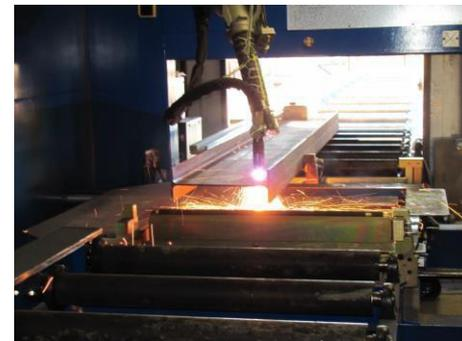
Roller system used to move material for fabrication
