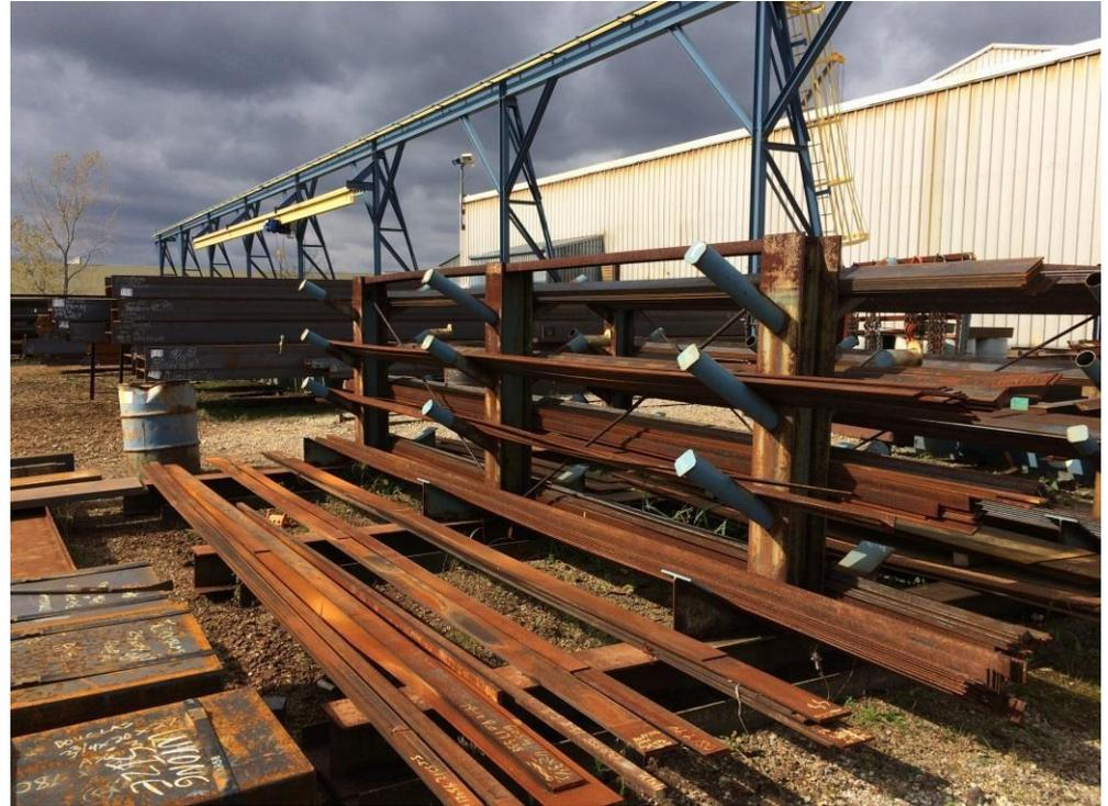
Racks used for storing plate and bar stock
