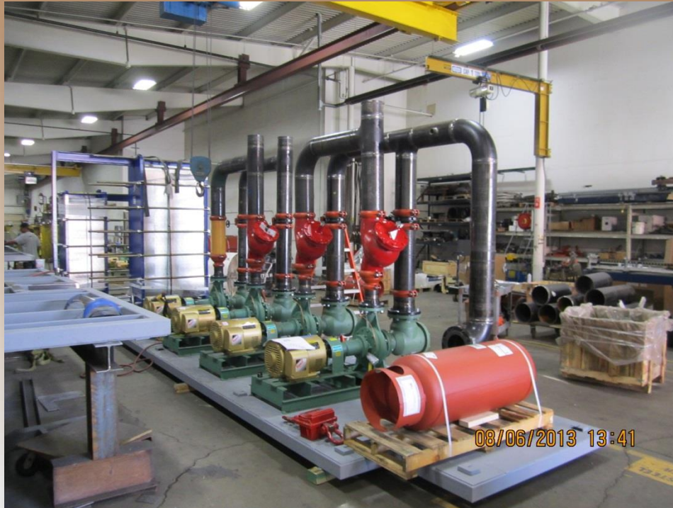
Prefabricated Pump Skids- Oakland University
