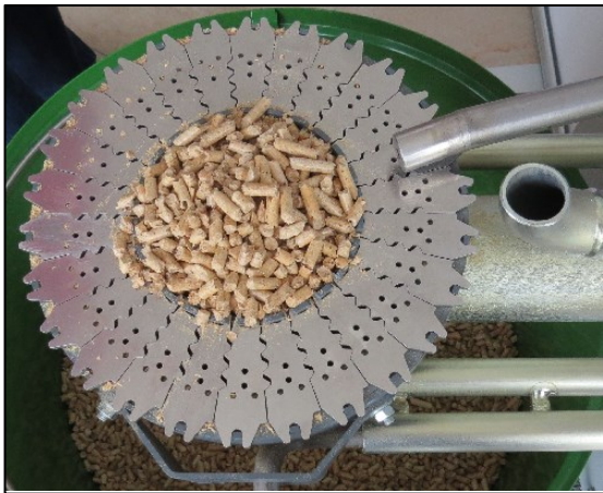
Wood pellets on a boiler burner plate.
