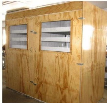
The oast includes two 4'x4'x8' cabinets with independent access doors and controls. Total capacity is 600 lbs wet hops which can be dried in 8 hours.
