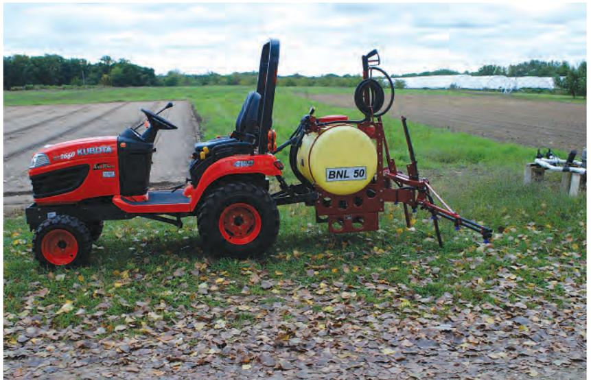
Versatile equipment is an economical means to get the job done with less labor. A sprayer for vegetable production allows liquid nutrient solutions such as fish emulsion or compost tea to be evenly applied to a field. Sprayers are also useful to apply OMRI approved pesticides. Note the versatility of this sprayer with a hand boom, which can be used to spray fruit trees or brambles.
