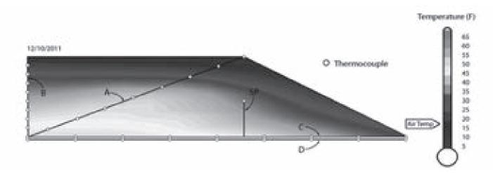
Figure 3. Temperature profile of Gera Road beet pile on December 10, 2011. Air temperature averaged 17 °F on this date. A, B, C, D and SP indicate five thermocouple harnesses; harness D was embedded approximately 2 inches into the soil. White circles indicate locations of individual thermocouples.
