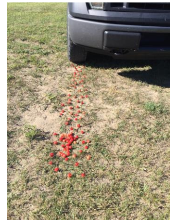
Figure 1. Driving over fruit to simulate mechanical crushing.
