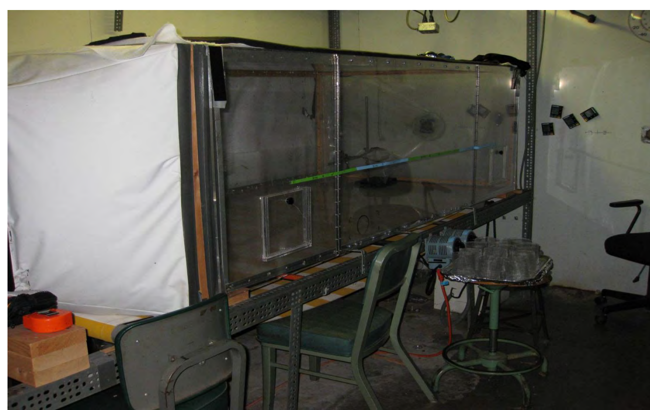
Figure 1: Wind tunnel (1.3 × 0.8 m in cross-section and 2.4 m long)
