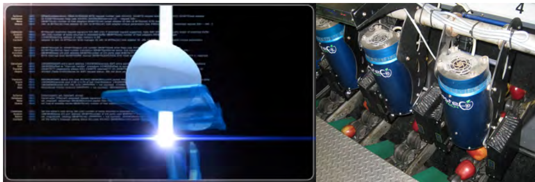
Figure 6. Images of Greefa (left) and Compac (right) technologies for internal defect detection and fruit sorting.
