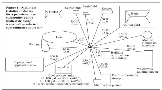
\*When siting any of these contamination sources from the well, one should not only consider isolation distance but also groundwater flow direction, geologic confining materials, casing depth, well pumping capacity, and any secondary containment design. For example, a fuel storage tank larger than 1,100 gallons, with secondary containment, may be sited 75 feet from a non-community public well.
