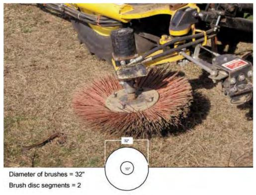
Typically, two 1" thick brushes are sandwiched between two 10" diameter metal plates. Brushing just below the graft unions of grafted vines
