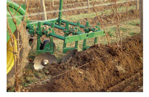
The practical concerns about building a unit of this type are that it must be durable and the torque created by this plowing action tends to steer the front of the tractor into the trellis area. Regarding durability, we constructed a heavy-duty frame on which we mounted these three disc plows. We have provided a schematic top view to show the dimensions of that framework.
