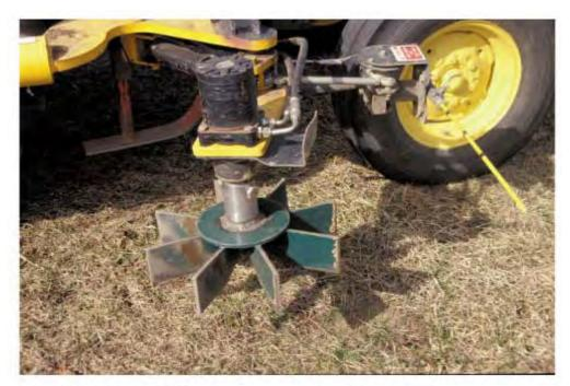
Overall diameter = 19 1/2" Height of a paddle = 4" Number of paddles = 8 Thickness of metal for paddle = 3/8"
