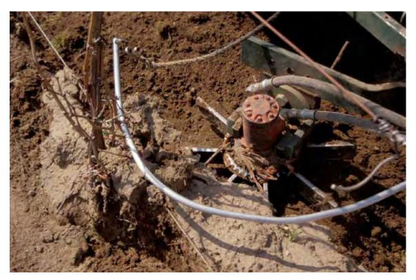
To complete the task of taking out the soil, a second implement was constructed consisting of 32" diameter brushes.
