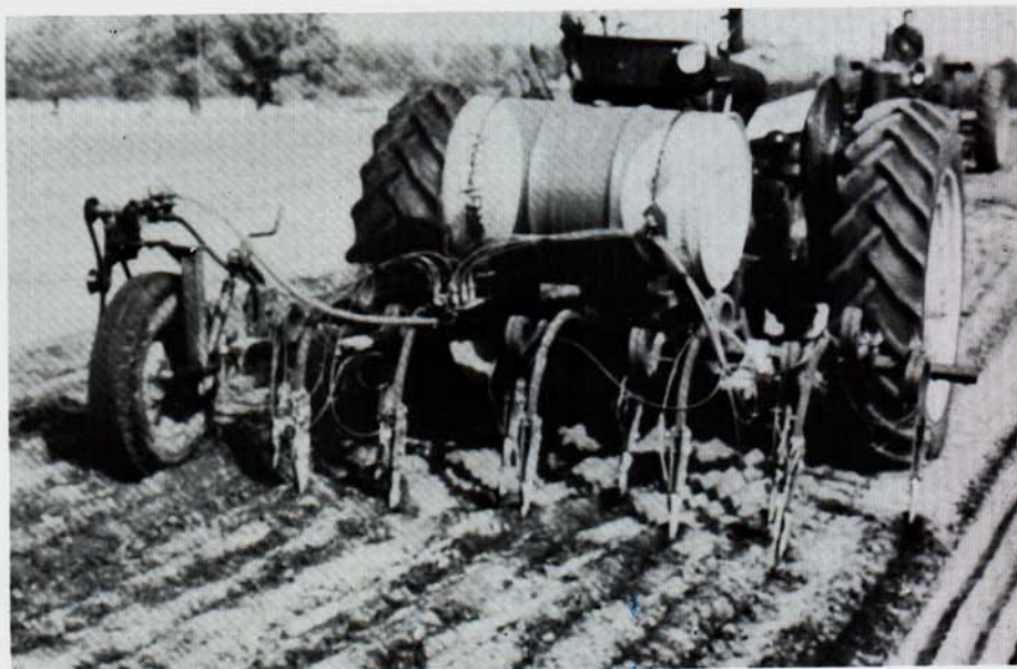
Figure 10. Injection of soil fumigant using a shank-type applicator.
