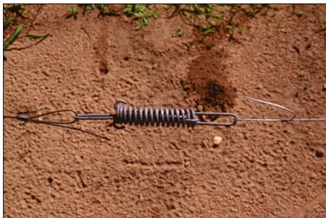
Fig. 5. This spring in a trellis wire absorbs changes in the tension of the wire due to temperature changes or crop load so that the wire itself does not exceed its yield point to become irreversibly stretched.
