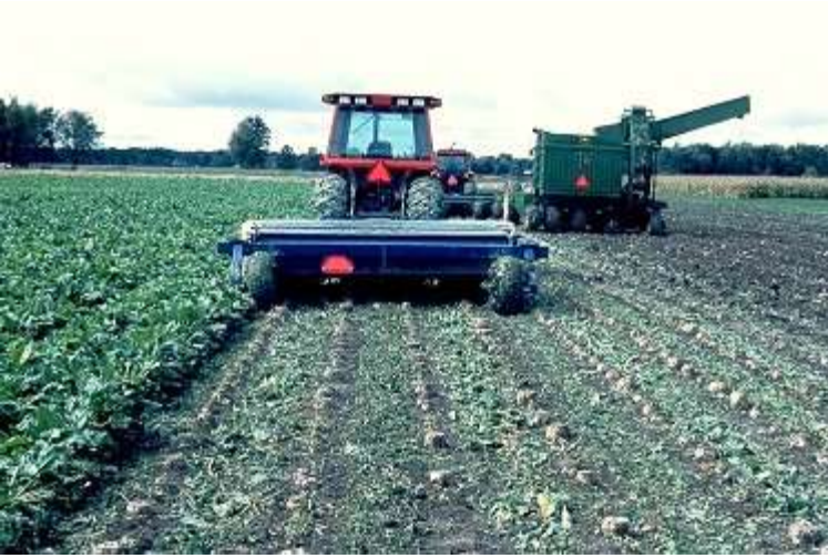
Beet leaves are removed prior to harvest with a rotating drum topper.
