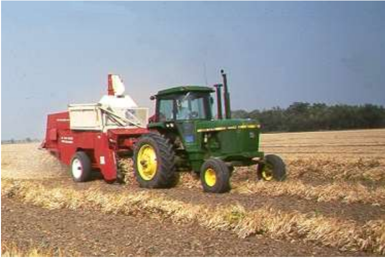
Beans are picked up in the field with either a pull type specialty combine or a modified grain combine and threshed.
