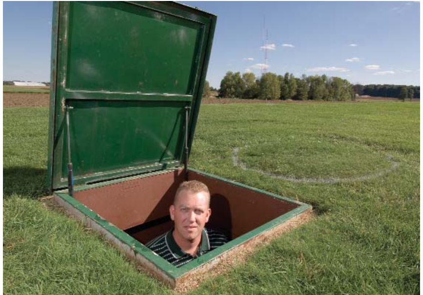
Kevin Frank, MAES turfgrass scientist, stands in a lysimeter that he uses to collect water runoff in his research on nutrient leaching. In his research, Frank has found that phosphorus is important for establishing a new lawn but not as important for an older one.
