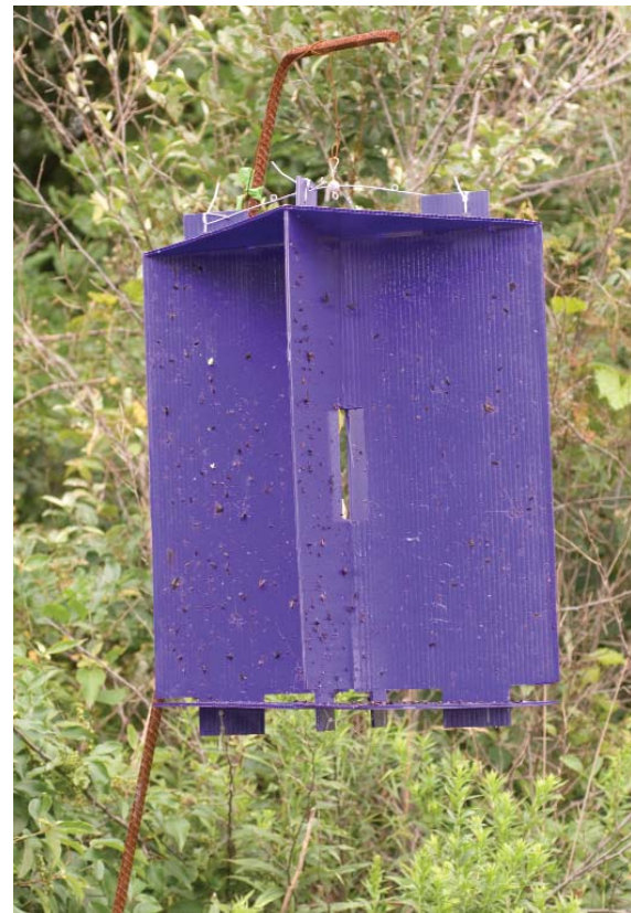
This box trap was designed by USDA APHIS scientists to test emerald ash borers’ attraction to certain substances. The box has a lure with ash volatile compounds inside and is coated with sticky material. If emerald ash borer beetles are attracted to the scent and/or the purple color, they get stuck on the trap.
