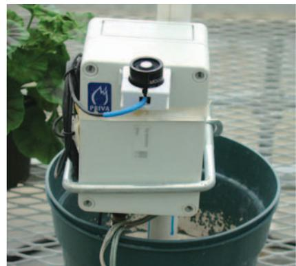
**Figure 4.** An external quantum sensor attached to a data-logging computer program.
