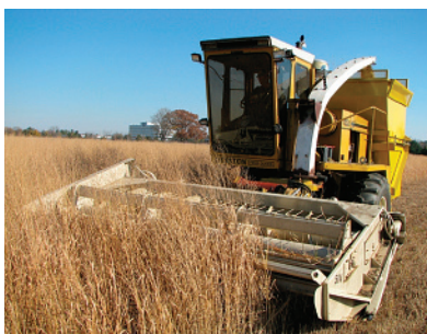
Harvesting senesced switchgrass with a modified Hesston forage harvester.
