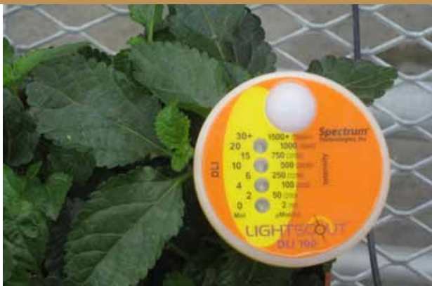
This is a small, mobile sensor without data logging capabilities.
