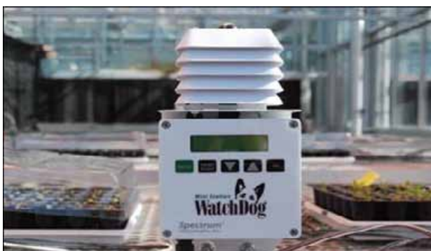
This is a mobile, self-contained data logger with a quantum sensor.
