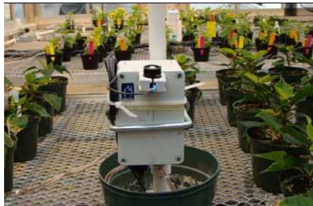
This is a quantum sensor that connects to a greenhouse environmental control system.
