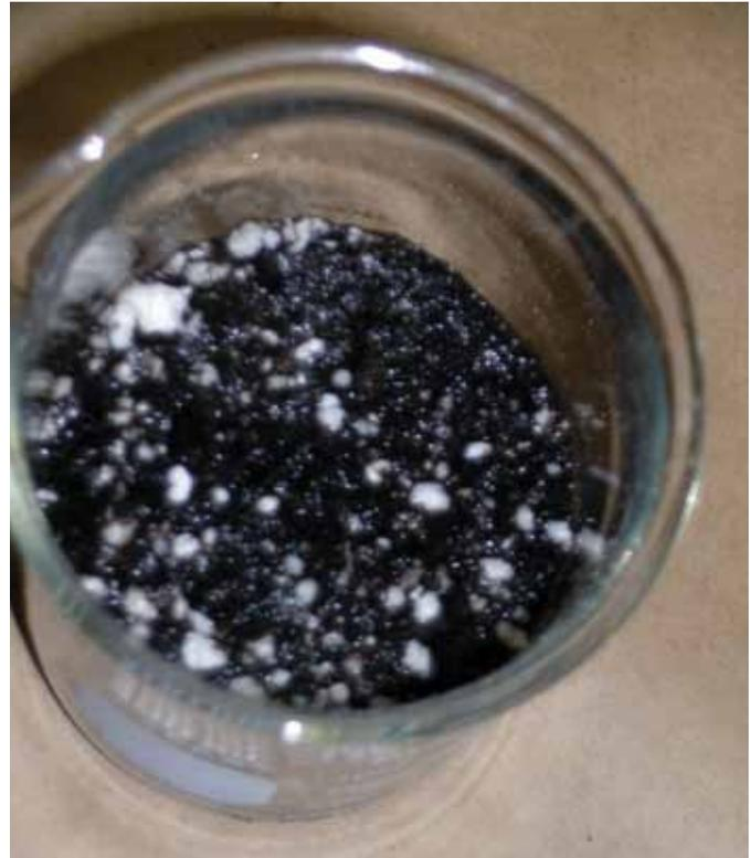
**Figure 3.** When using the saturated media extract method, the substrate should be saturated, but no free water should be visible on the sample surface.
