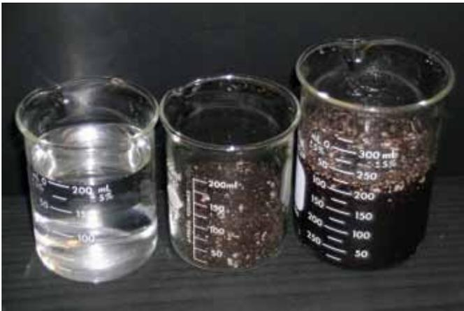
**Figure 5.** In the 1:2 dilution method, combine one part (by volume) of substrate with two parts (by volume) of distilled water.
