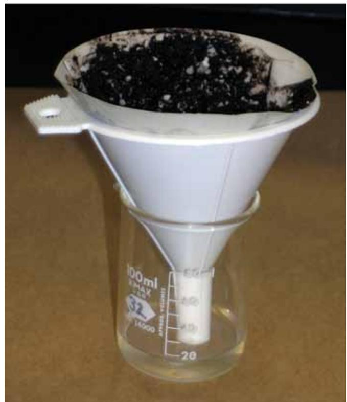
**Figure 4.** For the saturated media extract and 1:2 dilution methods, pour the samples into a clean funnel lined with filter paper or two coffee filters to collect the extract.
